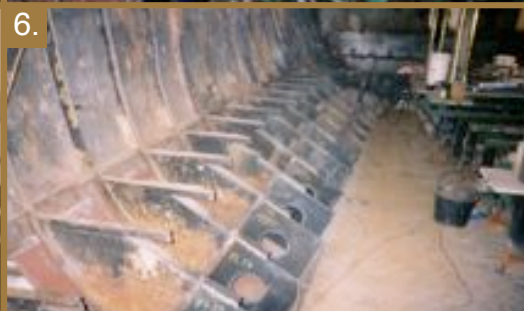
6. Structural stiffeners ensure Harmony II is fit for transatlantic travel.
