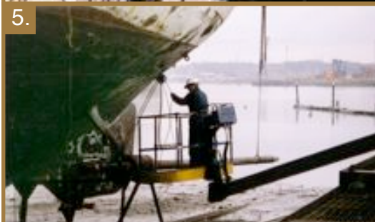
5. Prop shafts are removed at the stern of Harmony II.
