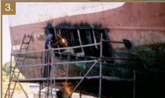
3. Welder cuts through the bow of Harmony II.
